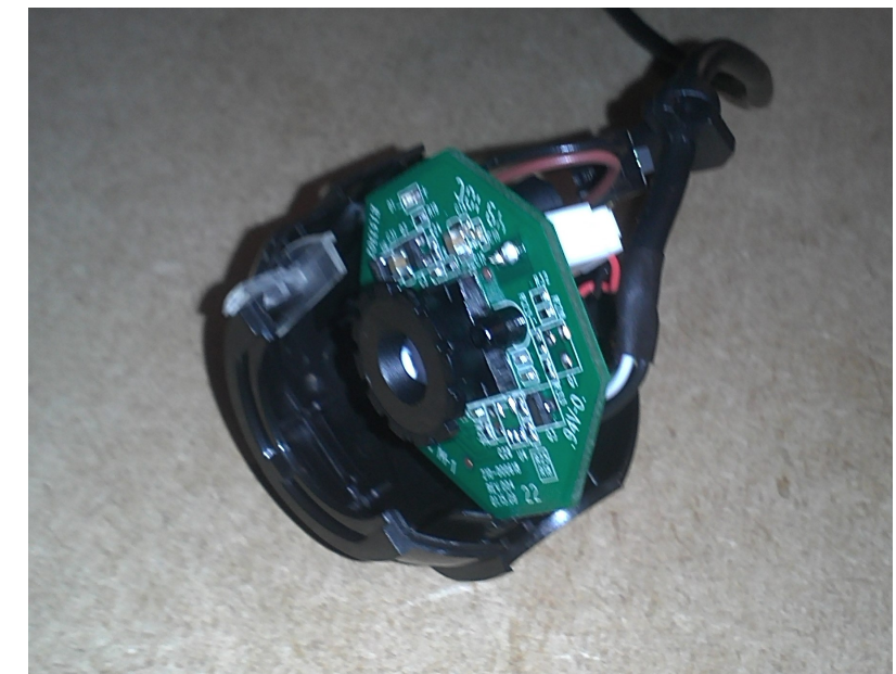
The PCB was then re-assembled and placed back in the camera casing.
