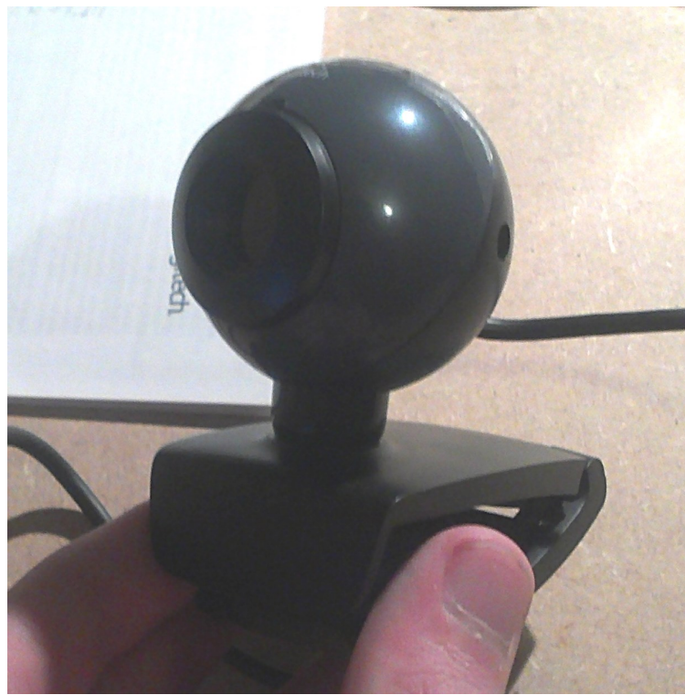
To create an IR camera I began with a simple 1.7 megapixel webcam
